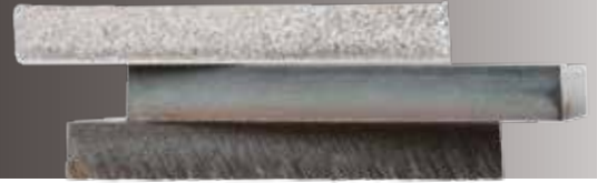
Relative cut performance on 12 mm mild steel
